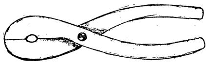
betonator Crimper used to crimp betonator on to Time Fuce: (made from 164. Hoop From) by Engineers to direct can over mine / lead coursed cable. mark on misde of wall. Exploser appointe Road mine (or Electric Bell when fractions). mies t- cables concealed under grand and brushed over with buch Hand Grenade
